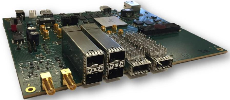
The Altera Arria SoC (10AS066-2E) based development platform is a network centric design with a single FMC mezzanine slot for application flexibility. All network and user interfaces are located on one edge and control / power on the opposite edge allowing for quick custom enclosure solutions. An integrated USB Byteblaster II is included for easy lab debugging.
